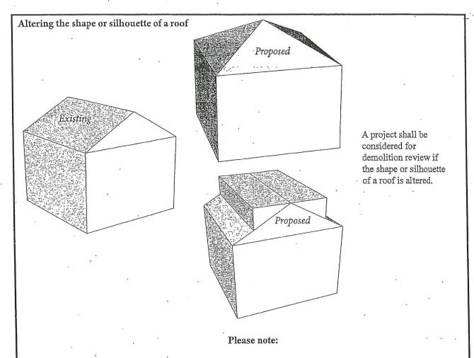
For the addition of dormers to an existing roof, if there is an indentation of at least one foot from both edges of a roof as well as at least one foot below the ridge and one foot above the eave of the roof, then the project may not be subject to review; or, if there is an indentation of at least three feet from the side edges of the roof and at least one foot above the eave of the roof, then the dormer may extend to the ridge of the roof without the project being subject to review.
