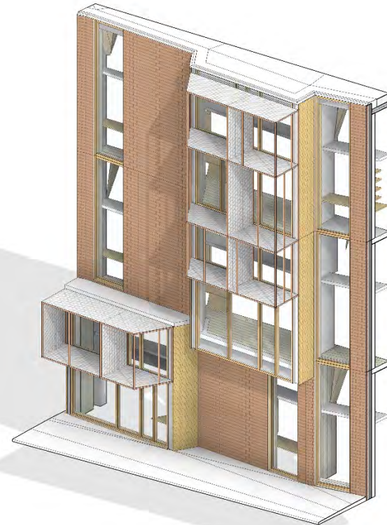
3D VIEW OF CLASSROOM FENESTRATION / SOLAR SHADING
